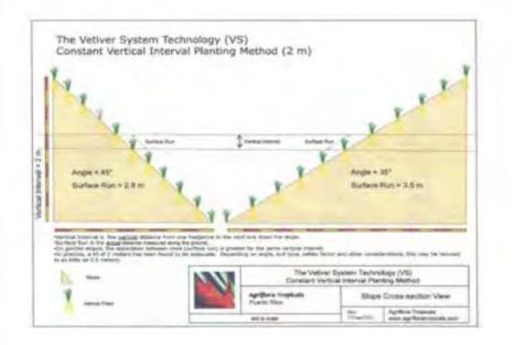
Design Principle of steep slope stabilisation with VS
